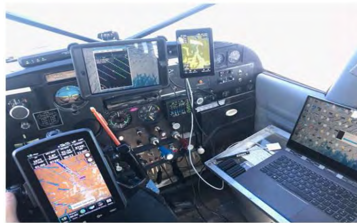
Cockpit view of Flight Management System with laptop controls necessary for software use
